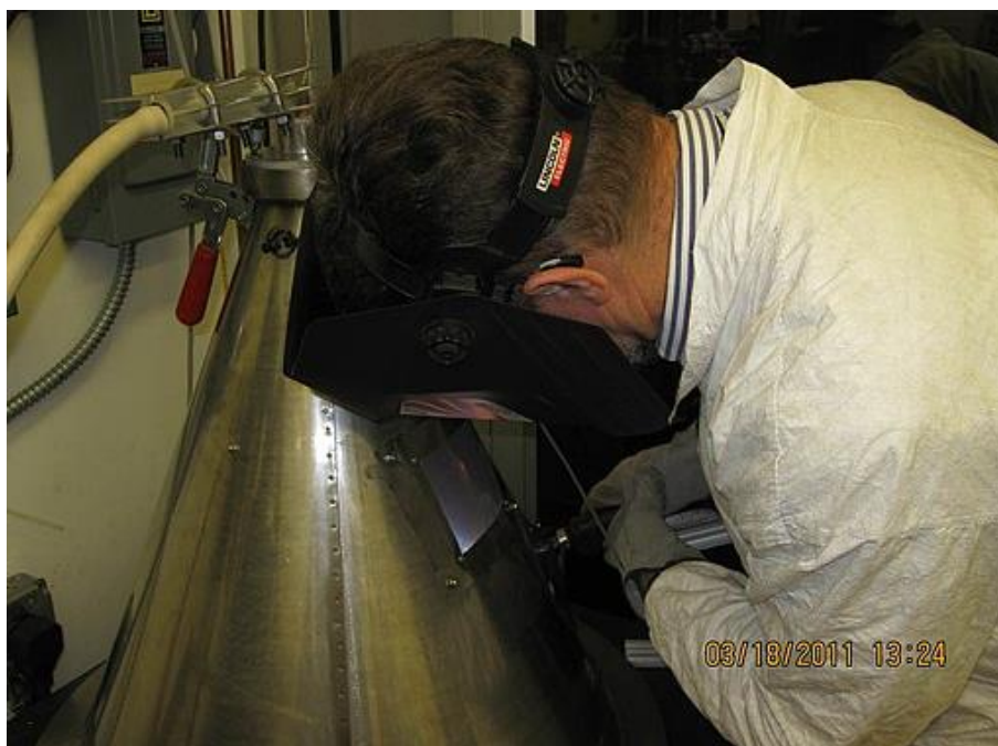
A person welding in an enclosed chamber to collect welding fumes for analysis and characterization. The goal is to identify and improve welding processes that generate as little fume, especially hexavalent chromium, as possible while maintaining good quality welds. (National Institute for Occupational Safety and Health, 2011)
